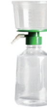
REF BS6344902-1000ML PES membrane, Sterilized Diameter: Ø90mm, Pore size: 0.45µm Funnel capacity: 500mL Receiving bottle capacity: 1000mL 1 Piece/pack, 12 packs/case
