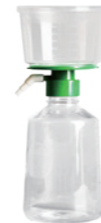
REF BS6342902-1000ML PES membrane, Sterilized Diameter: Ø90 mm, Pore size: 0.22µm Funnel capacity: 500mL Receiving bottle capacity: 1000mL 1 Piece/pack, 12 packs/case
