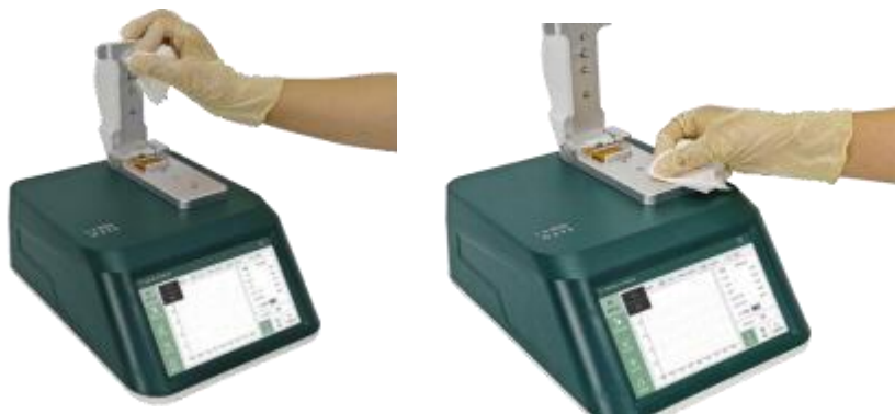
Figure 3.4 Cleaning Residual Samples from the Upper and Lower Bases
